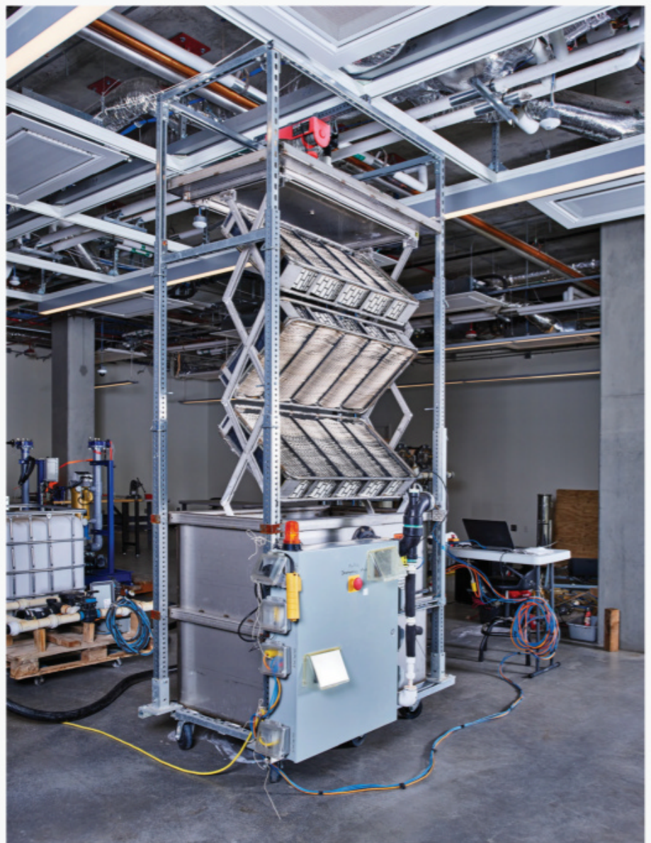
An artificial tree designed by Klaus Lackner of ASU sucks CO 2 from air that moves through the device.
